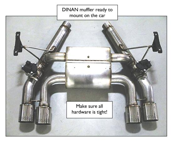
9. Place exhaust clamps provided in the hardware kit onto the ends of the stock exhaust pipes. With DINAN exhaust secured on a jack or stand, put the muffler in place. When mounting the muffler it should be held with the tips up near the bumper and the muffler pushed forward against the ends of the stock pipes.
