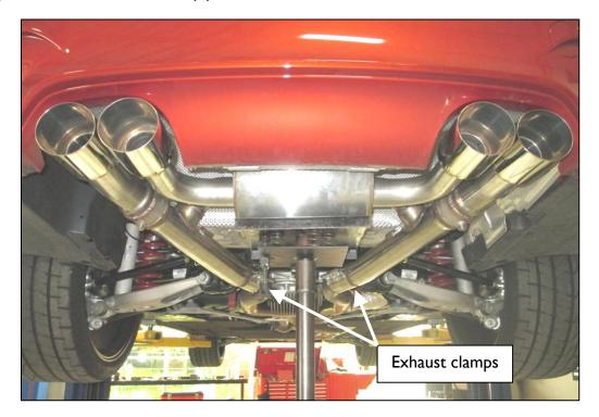
Mount both muffler hangers using the stock mounting nuts that were saved from removal of the stock muffler. Torque the nuts to 14 ft-lbs (19 Nm).
