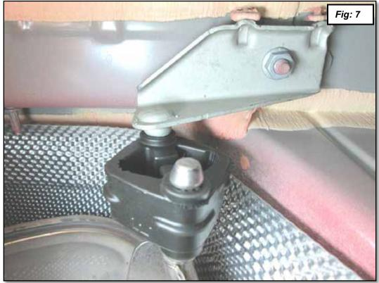
7. Transfer muffler hangers to new mufflers. Replace rubber hangers as needed. Lift the new muffler into the car and bolt the hangers into place. Torque the hanger nuts to 19Nm.
