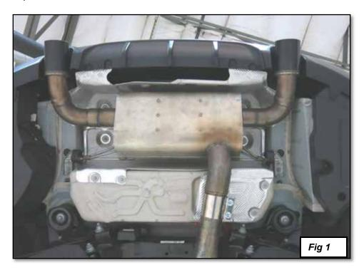
2. Unplug the wire harness from the exhaust flapper valve on the driver's side of the stock muffler. Remove the three screws holding the valve actuator to the valve. Remove the wire from the clips holding the wire to the side cover.
