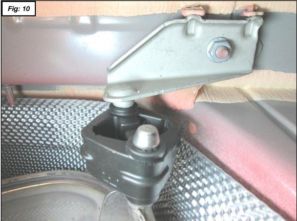
9. Transfer muffler hangers to new mufflers as shown in figures 11 and 12. Replace rubber hangers as needed.
