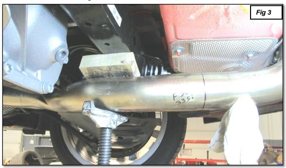
4. This step applies to F32 435i and xDrive only; skip to step #6 if you are working on a F30/F34 335i. For a 435i find the BMW factory punch mark on the exhaust. Measure ¾ of an inch from the punch mark toward the back of the car and cut at that point.
