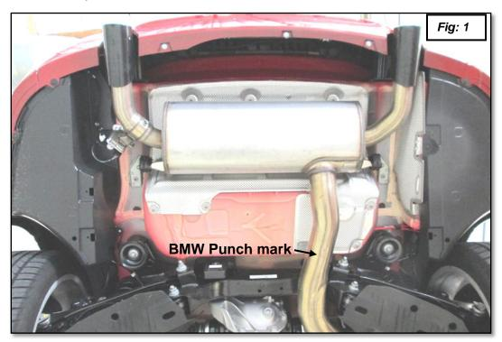
2. This step applies to F30/F34 335i and xDrive only; skip to step #4 if you are working on a F32 435i. For a 335i cut off the stock muffler at the punch mark as shown in figures 1, 2and 3. Mark the cut line.
