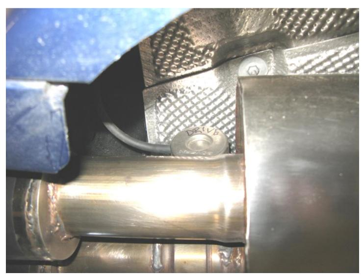
12. Visually inspect the muffler. Check for at least  $\frac{1}{2}$ " clearance in all areas. You can bend the heat shields slightly if needed.
