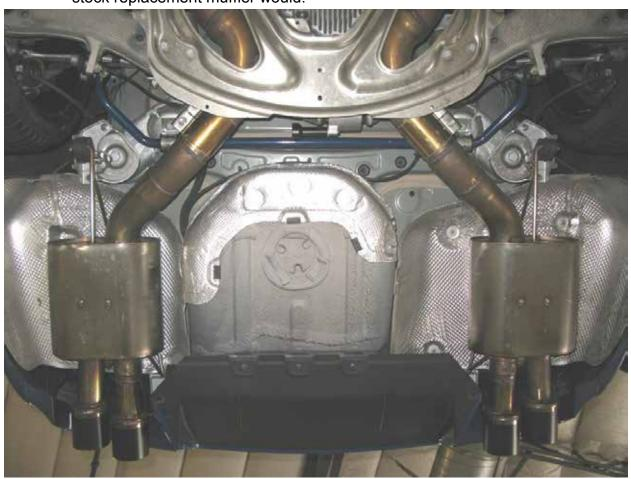
2. Cut off the stock mufflers at the punch marks as shown in figures below. Mark the cut line. Use a Sawzall or similar cutting tool.
