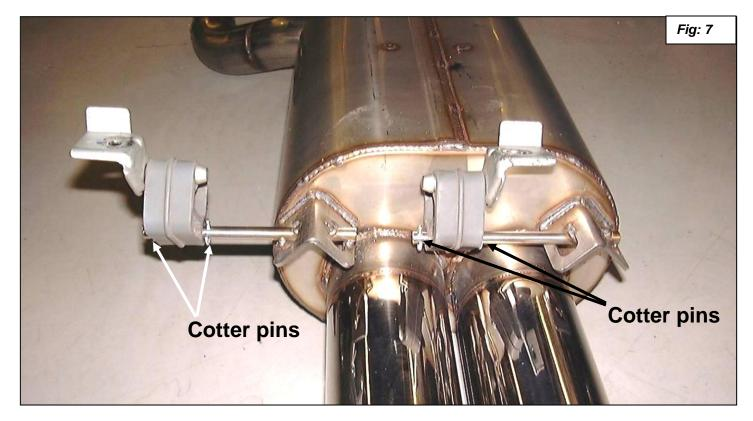
8. Install the front hangers onto the mufflers as shown in figure 8. Install a cotter pin in the outer hole only. Bolt the ground strap as shown.
