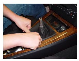
3. Lift up and remove shifter isolation boot.
