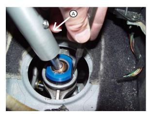
12. Replace selector arm through bottom of shifter. Place included washers on either side of Dinan shifter. Replace U-clip.
