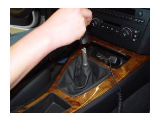
2. Squeeze together the sides of the shift boot and lift up to remove.
