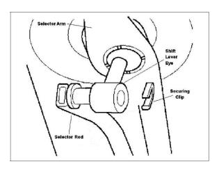
6. Spread the jaws of needle-nose pliers apart so that the tips fit in opposing slots of the plastic ball-clamp. Rotate 1/4 turn clockwise.
