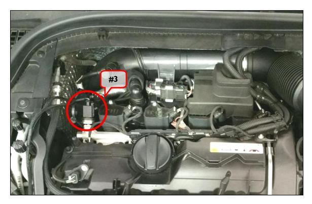
12. The fuel rail pressure sensor connection could be one of two configurations. Please examine your harness connector and compare it to the photos below. <u>One style is a D-shape, while the other style is an oval-shape.</u> If you do not have the correct harness for your vehicle, please contact Dinan for an exchange -- do not continue with installation
