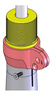
12. Install the spring perch and black plastic isolator disc (in Coil-Over Hardware Kit) as shown. Adjust the perch to about 1/2" up from bottom. This will be the starting ride height setting, and should get you very close to Dinan's target bumpstop clearance measurement. Snug the 6mm screw to lock the perch into place.
