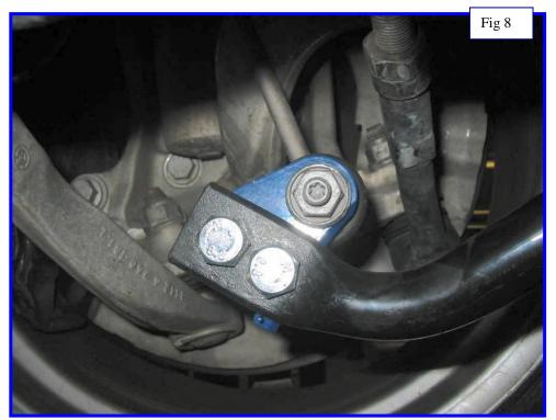
9. Bolt the drop link in hole #I and torque to factory specs. Repeat for other side. (See Figure #8)
