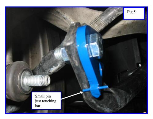
6. Once you have the bolt tight and it resembles these photos, take the 10mm drill bit supplied in the kit and drill just enough through hole #3 to get a good center mark on the bar. Next use a smaller bit (approx. 3/16") to drill a pilot hole in that spot. Step up one more time (approx. a 5/16" bit) before you finish with the 10mm bit. If you try to drill thru the bar in
