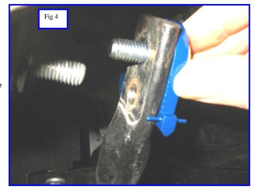
5. Next use the 10mm plain nut to fasten the plate to the bar. As you tighten the bolt, rock the plate over until the small pin just hits the side of the bar. This will line up Hole #3 so you can drill the bar for it. (See Figure 5)
