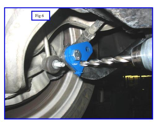
one step with the 10mm bit, you will burn up the bit. Make sure the plate does not move during drilling. (See Figure 6)
