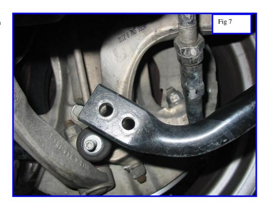
8. Now bolt the plate back on the **OUTSIDE** of the sway bar using the supplied bolts and lock nuts. This is opposite of how you had it on to drill the holes. The bolts are a close together so you may need to use hand wrenches to fully tighten them. These bolts must be securely attached to prevent loosening and poor handling.
