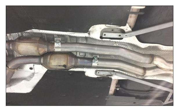
10. Slide the 2 muffler clamps forward onto the midpipe and reinstall the clamp hardware.
