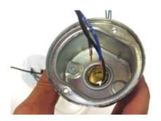
2 Feed the brown and blue wires through the holes on the included grommet. Carefully slide the grommet up over the lamp socket.
