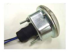
Align the LED board into position in the housing and place the gasket on top as shown in the photos below. Re-install the lens.
