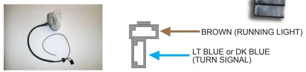
Male blade terminals and connectors are included in case your factory front light harness connector is missing or damaged.
