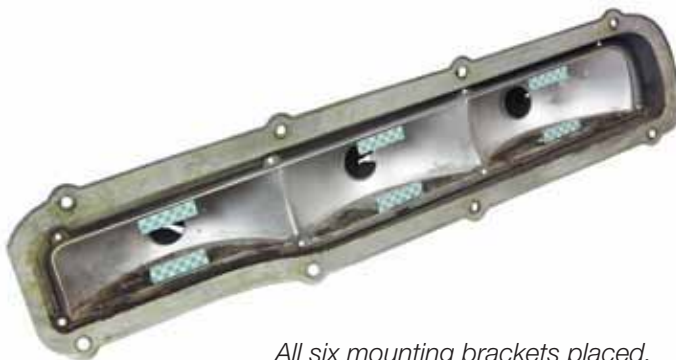
All six mounting brackets placed.
