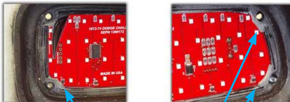
LED panel sits on the housing ledge. Some trimming of the gasket may be required.
