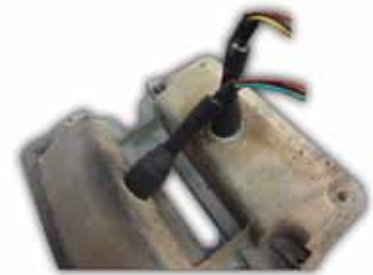
2. Shrink tube shut the wires to the boot.
