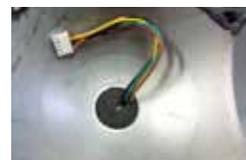
The slide switch is accessible through the light socket hole. This allow you to change the LED setting to standard or sequential without taking out the LED panels.
