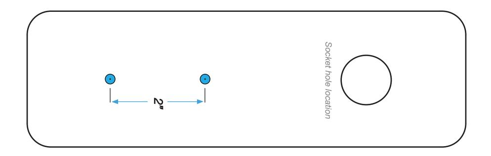
1. Cut out the template and position it on the inside of the housing, matching the light socket location.
