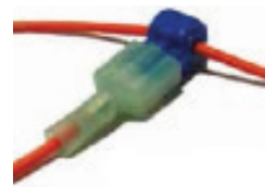
3. Plug connector into T-Tap
