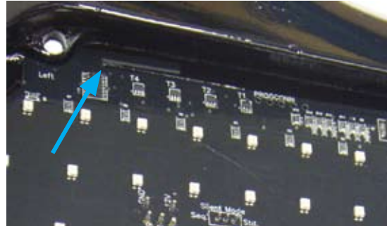
Arm portion sitting in gasket groove.
