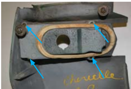
Location of 4 screws that hold the chrome bezel on.
