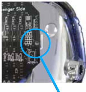
LED panel mounting hole.
