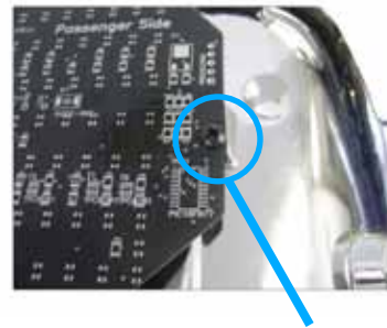
Lightly fasten screw.
