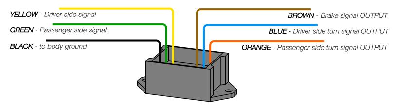
The DIGI-TAILS Taillight Signal Separator will convert the Passenger and Driver signals with no dedicated brake light signal and output a driver side turn signal, passenger side turn signal, and Brake light
