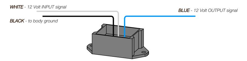
The DIGI-TAILS Brake Light Pulse will convert the any 12 volt signal (like a 3rd brake light signal) and quickly pulse the output ON/OFF 3 times.
