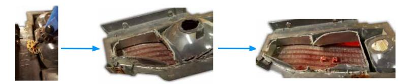
6. Be sure that the cut at the bottom of the bucket is even with the housing ledge.
