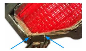
**8.** Below is the housing fully trimmed up. All cuts are at or below the housing ledge to allow the LED panel to sit in place with out issue. Clean out any dust and plastic debris.
