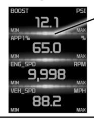
The separator lines will change from Red to **Green**, which indicates that the device is actively **recording** (datalogging).
