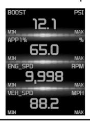
**STEP 2 -** Press the OK button to begin recording the PID data. Press the OK and follow the steps. button again, to stop the recording.
