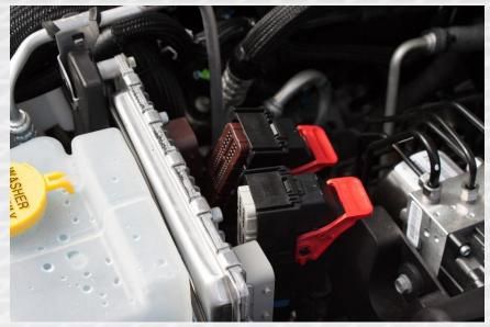
3. Using a 10 mm wrench/socket, remove the 3 bolts holding the PCM to the bracket behind the driver's side headlight. Take note that one of these bolts is securing a ground cable that must be reconnected.
