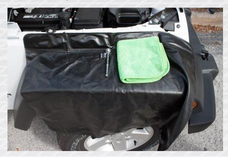
1. Disconnect/remove negative terminal from the battery using a 10 mm socket.
