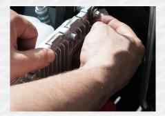
6. Remove upper PCM connector first by pressing center button and sliding lock back words away from the computer wiggle if tight do not force red clip. Follow this by the bottom connector.
