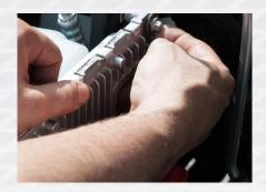
4. Remove upper PCM connector first by pressing center button and sliding lock back words away from the computer wiggle if tight do not force red clip. Follow this by the bottom connector.
