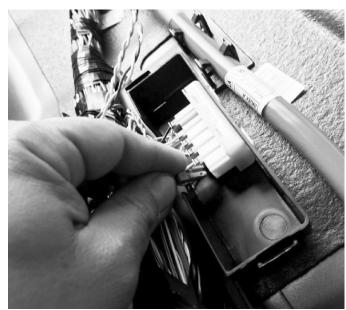
STEP 5 - Insert the White Plug into the green module socket as shown. (Any available slot will work.)
