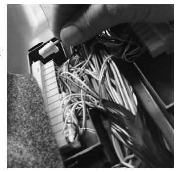
step 6 - Snap and re-secure the module cover. Route the power and ground cables toward the battery as shown.
