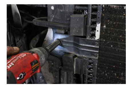
2. Once all four bolts are removed, remove all the torx headed screws holding the four brackets onto the condenser. To get to the bottom screws you will have to lift the condenser up slightly.
