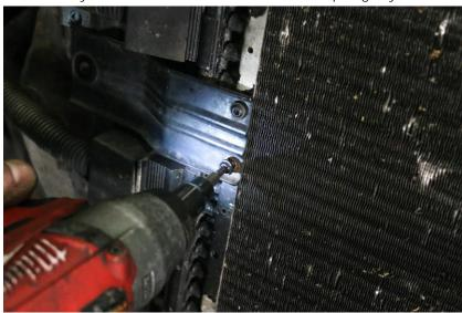
3. Place the condenser cover onto the condenser. Reinstall the four brackets with the factory torx screws. Make sure as you tighten the torx screws the mounting hole for the 13MM bolts line up.
