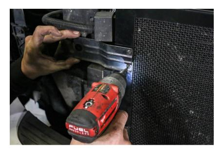
4. Reinstall the four 13MM bolts. Note: Some condensers may not use all three screws in the bottom brackets as shown below.
