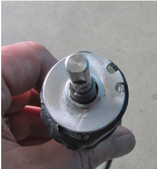
Figure 7 - Wiper Switch Clocking Spacer
