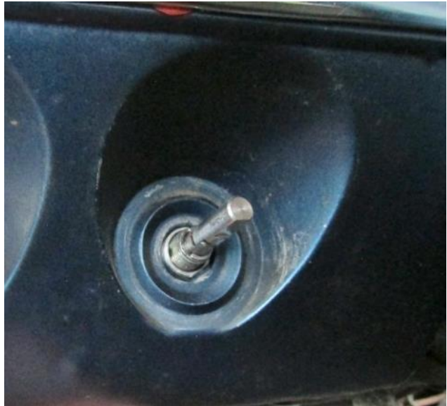
Figure 8 - Install Wiper Switch
