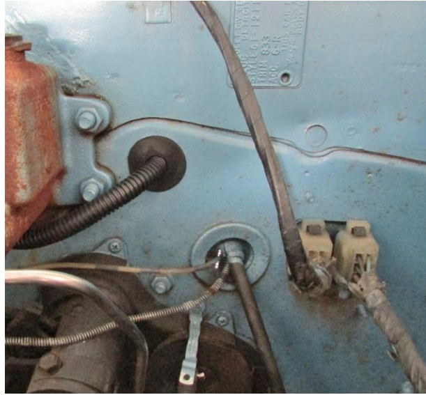
Figure 14 - Install Wiper Motor Harness
