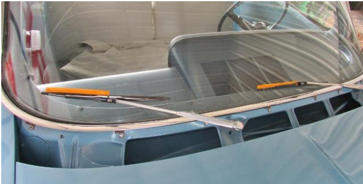
Figure 1 – Remove Wiper Arms & Cowl Panel
