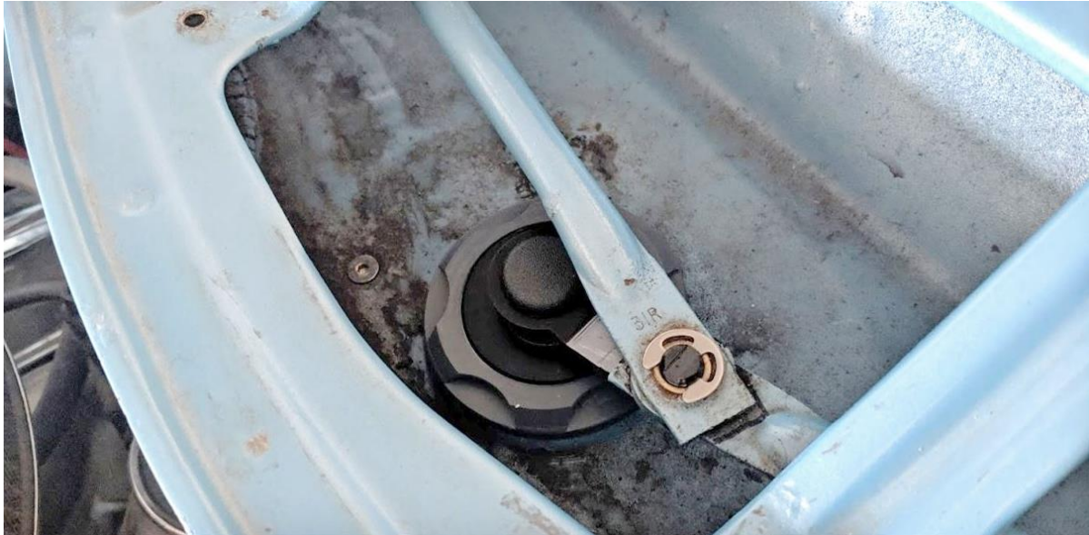
Figure 5 – Attach Wiper Linkage to Pitman Arm
