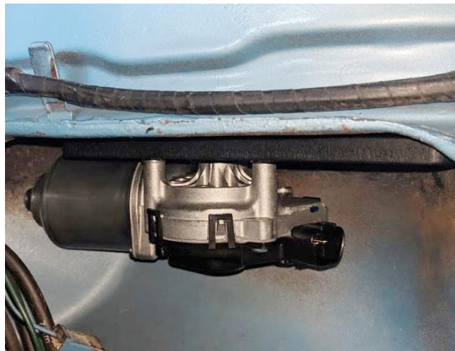
Figure 3 - Mount Wiper Motor
