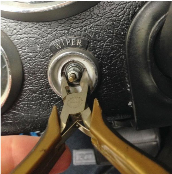
Figure 16 - Remove Switch Nut
