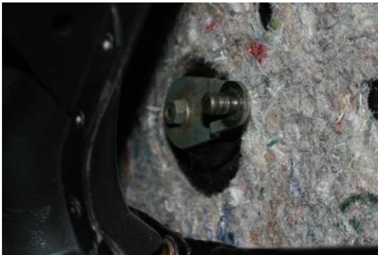
Figure 6 - Remove Wiper Linkage
