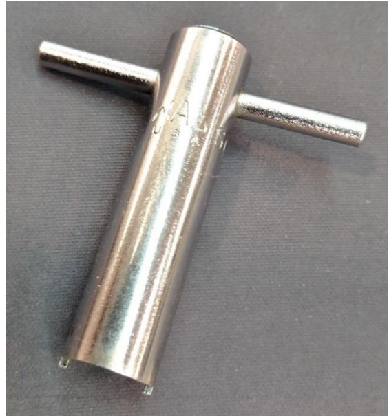
Figure 17 - Wiper Switch Removal Tool
