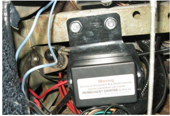
Figure 28 - Mount Control Module Bracket
