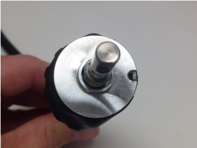
Figure 18 - Wiper Switch Clocking Spacer
