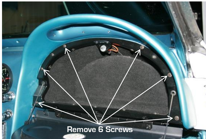
Figure 3 - Remove 6 Mounting Screws
