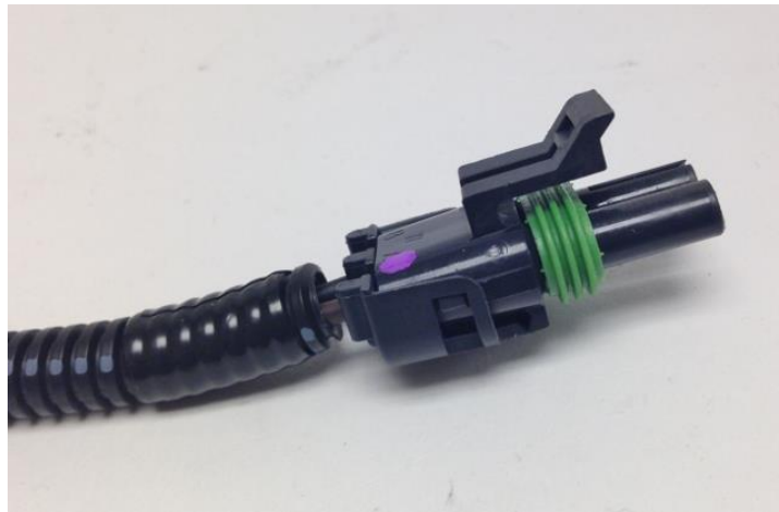
Figure 25 - Washer Pump Connection
