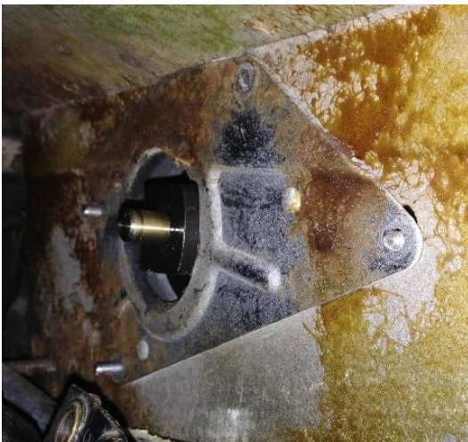
Figure 12 - Mount the Wiper Motor
