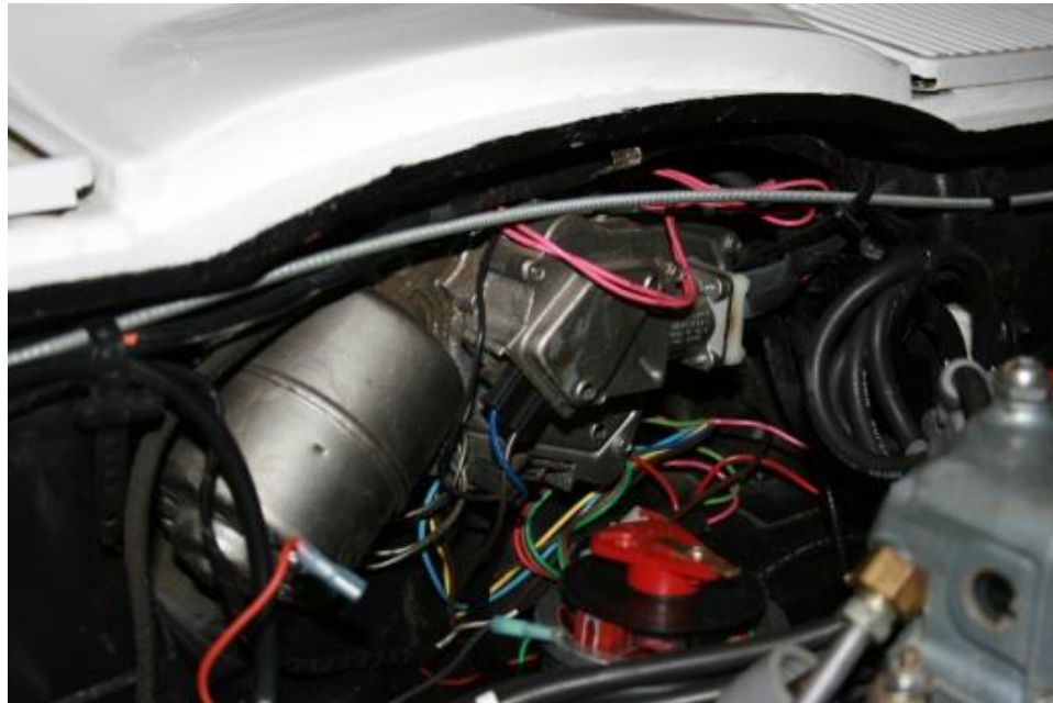
Figure 1 - Remove Distributor Cap
