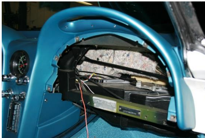
Figure 4 - Remove Glove Box
