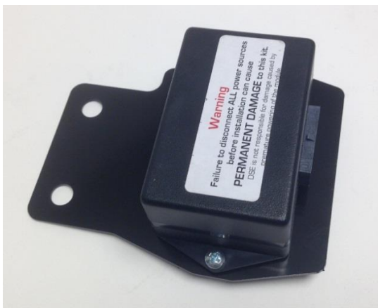
Figure 26 - Wiper Control Module & Plate Module
