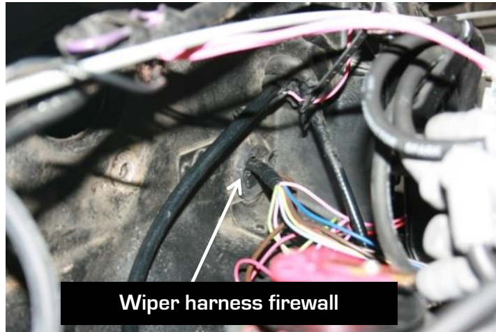
Figure 8 - Remove Firewall Grommet
