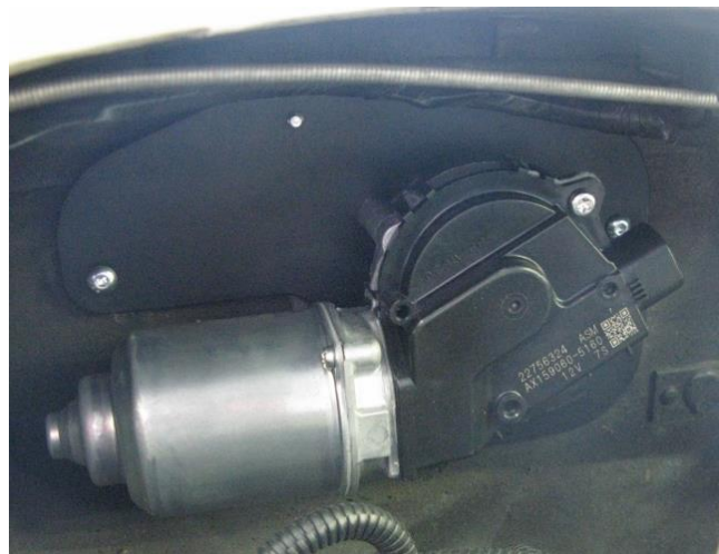
Figure 12 - Mount the Wiper Motor
