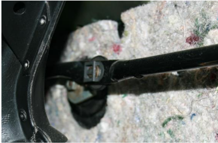
Figure 5 - Remove Retaining Clip
