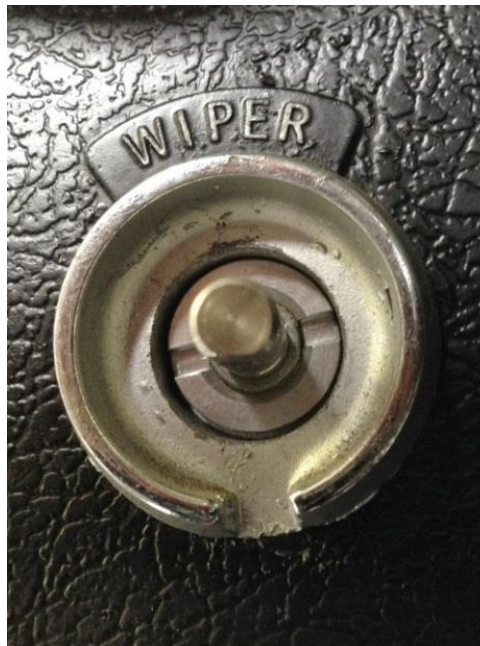
Figure 20 - Install Switch Nut
