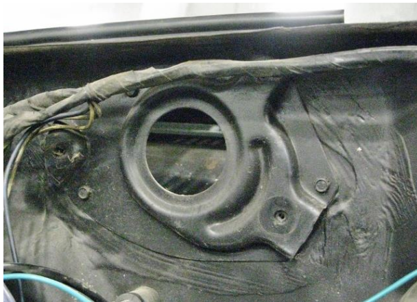
Figure 1 – Remove Factory Mounting Plate
