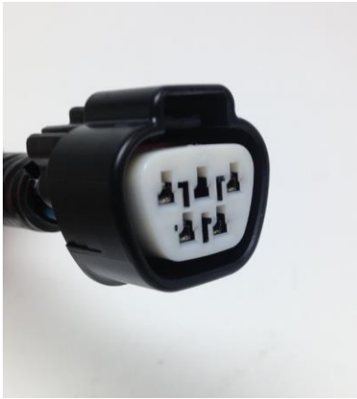
Figure 6 – Wiper Motor Connector
