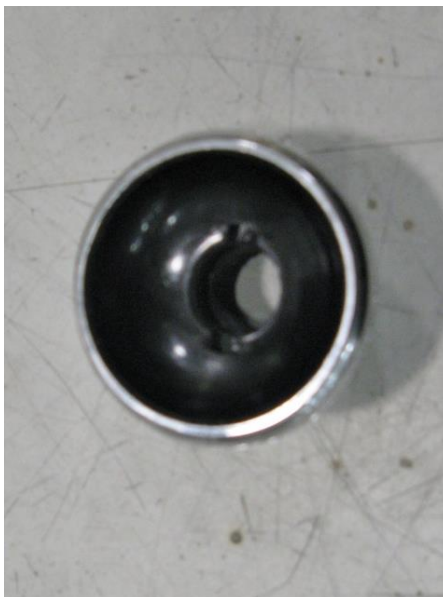
Figure 3 - Wiper Switch Retainer/Bezel
