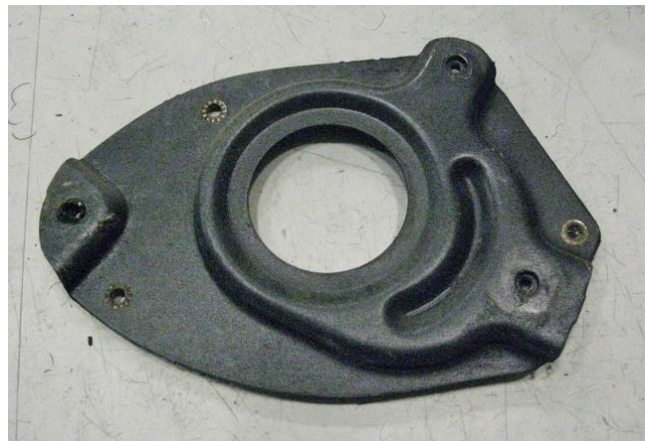
Figure 1 – Remove Factory Mounting Plate
