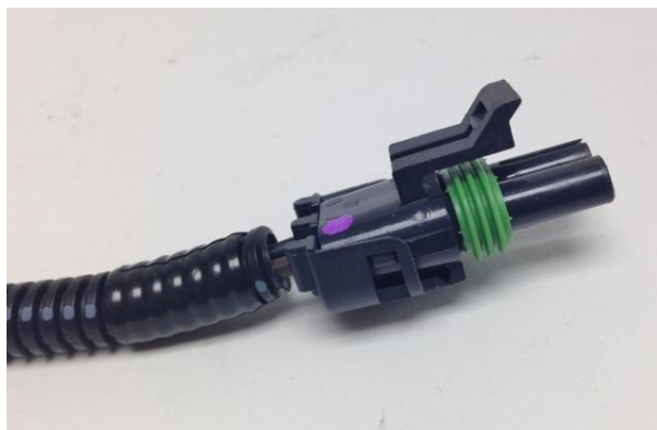
Figure 8 – Washer Pump Connection
