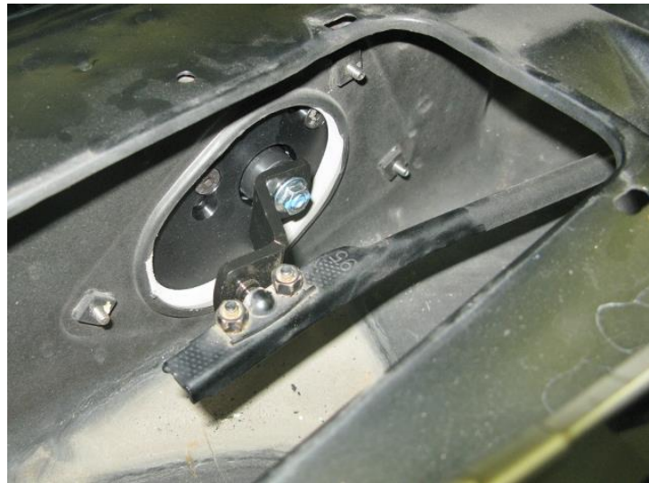
Figure 11 – Attach Pitman Arm to Wiper Linkage
