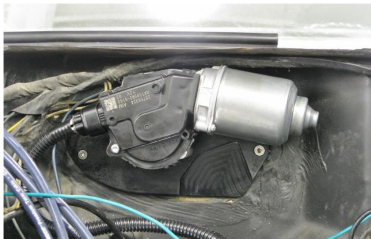
Figure 7 – Install Wiper Motor Connector
