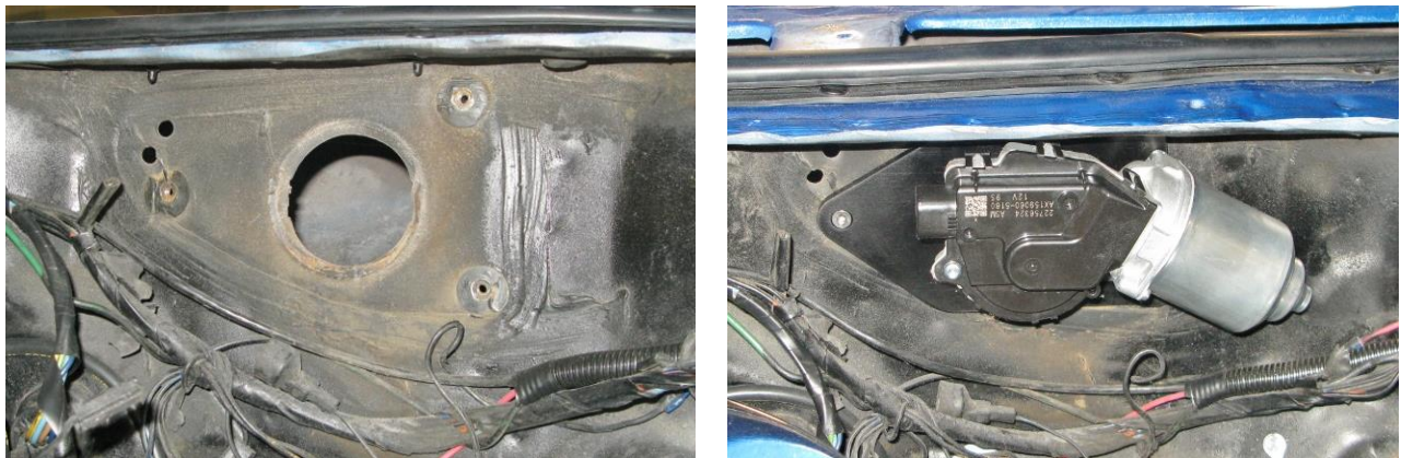
Figure 2 - Wiper Motor Orientation (1970-72 Mounting Plate Shown)
