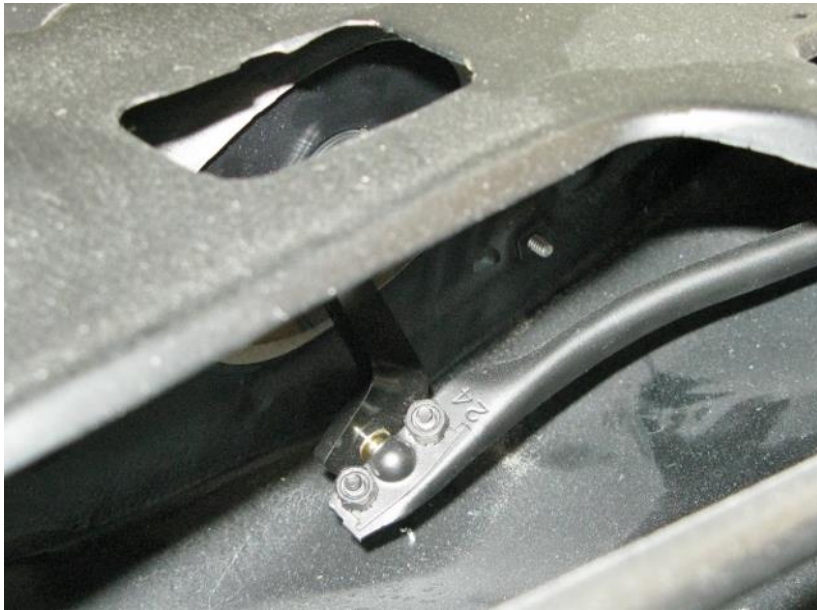
Figure 2 - Attach Pitman Arm to Wiper Linkage
