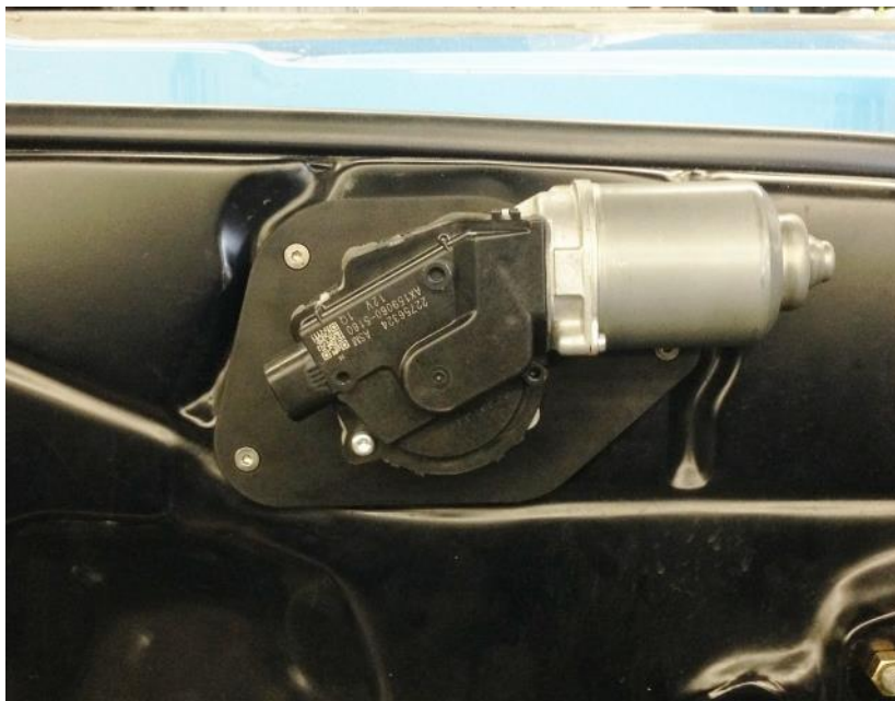
Figure 1 - Attach Wiper Motor to Firewall
