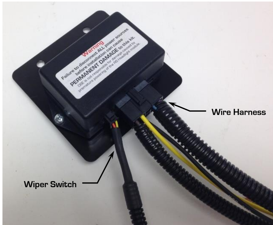
Figure 8 - Connect Wiper Switch & Harness to Module
