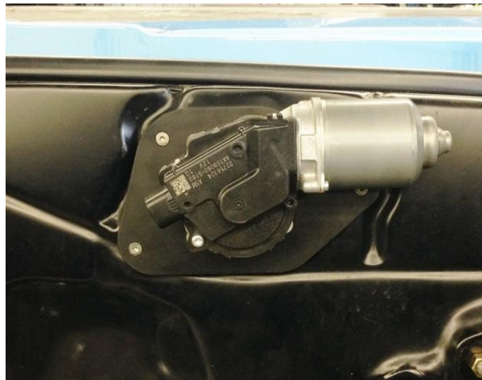
Figure 2 - Attach Wiper Motor to Firewall
