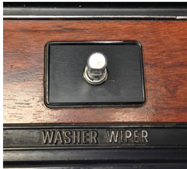
Figure 10 - Install Wiper Switch & Alignment Plate
