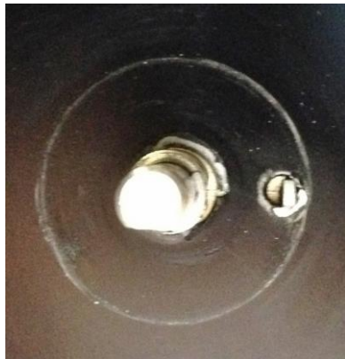
Figure 6 - Install Wiper Switch
