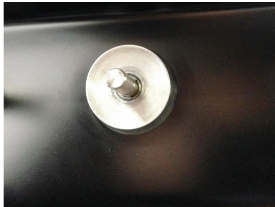
Figure 7 - Thread Bezel onto Switch
