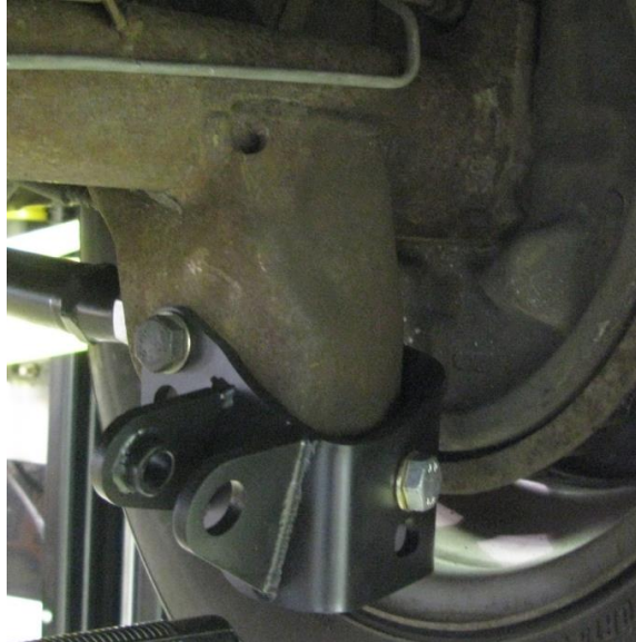
Figure 1 - Installed Lower Coilover Bracket (P/N: 042420 Shown)
