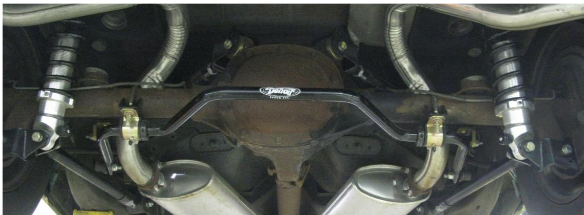
Figure 3 - Completed Coilover Installation
