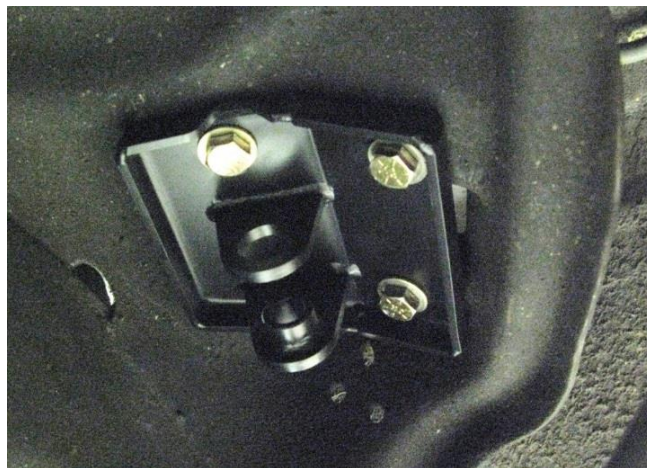
Figure 2 - Installed Upper Coilover Bracket
