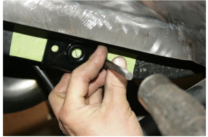
Figures 5a and 5b – Locating the Anti-roll Bar Mounting Bracket Holes on the Framerrail
