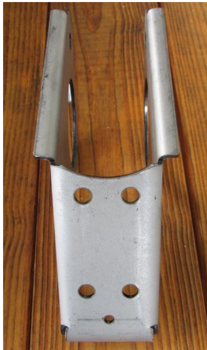
Figure 1 - Pre-Drilled Holes in Coilover Bracket
