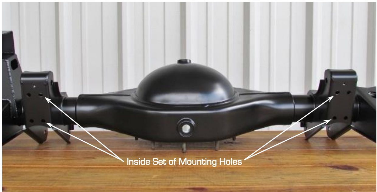
Figure 9 - Use the Inside Set of Holes to Mount the ARB Bracket
