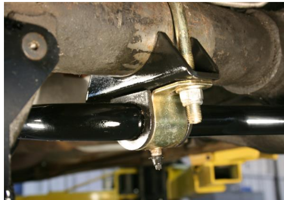
Figure 4 - Anti-Roll Bar Mounted on Rear Axle
