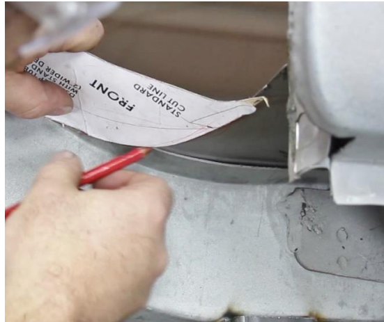
Figure 17 - Connect Frame Rail to Inner Tub Cut-Out
