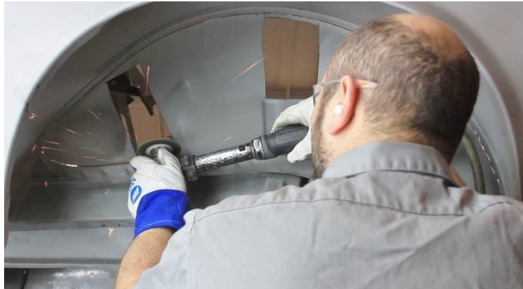
Figure 6 - Cut Out & Remove Inner Tub
