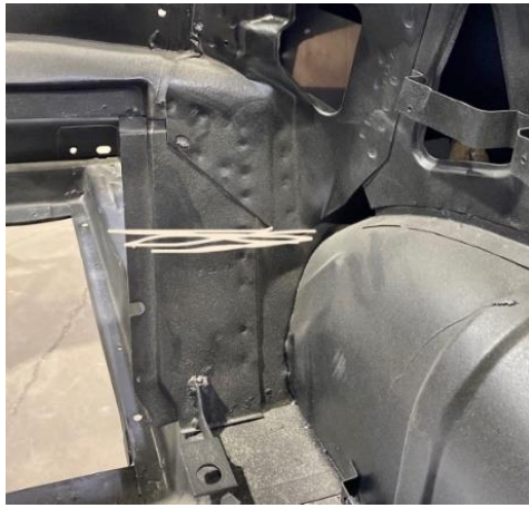
Figure 3b - Remove Seat Support (1965 Fastback)
