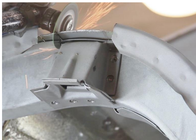
Figure 8 - Remove Bump Stop Bracket
