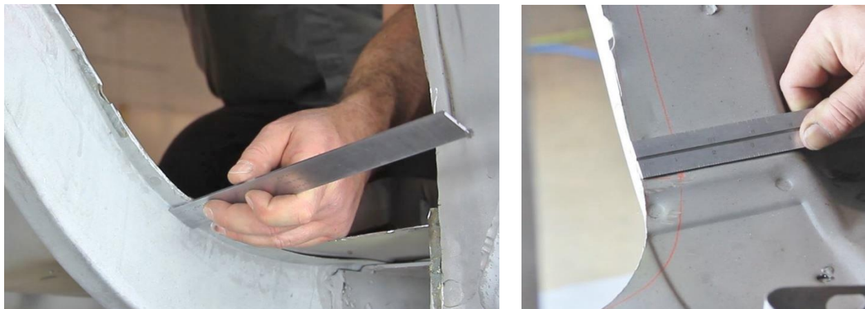
Figure 18 - Transfer Flange Dimension
