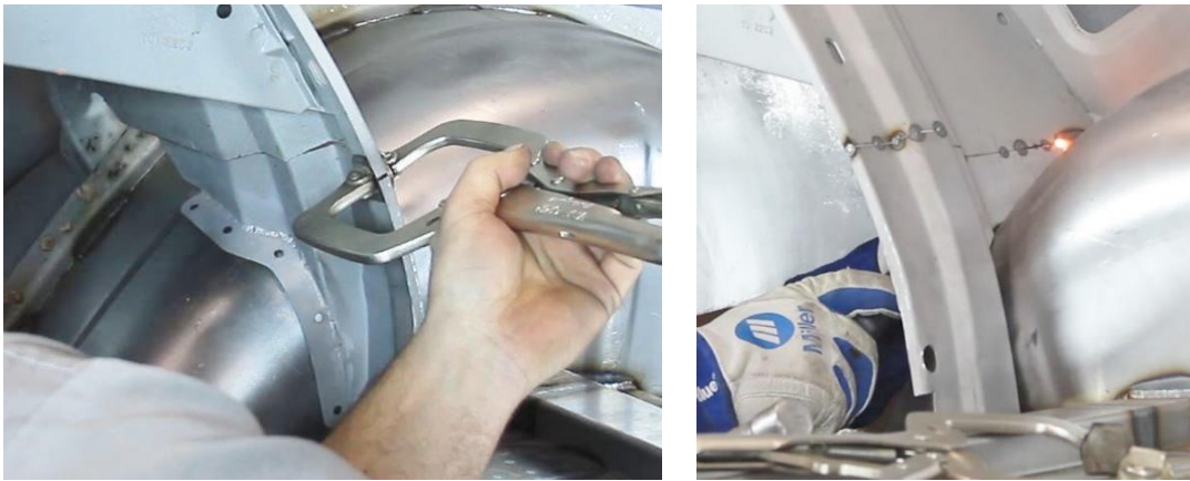
Figure 29 – Weld Rear Seat Support to Mini-Tub [Fastback]
