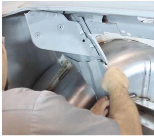
Figure 28 – Modify Rear Seat Support
