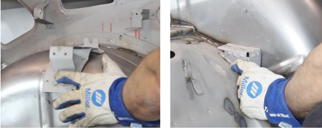
Figure 31 - Re-attach Upper & Lower Seat Brackets
