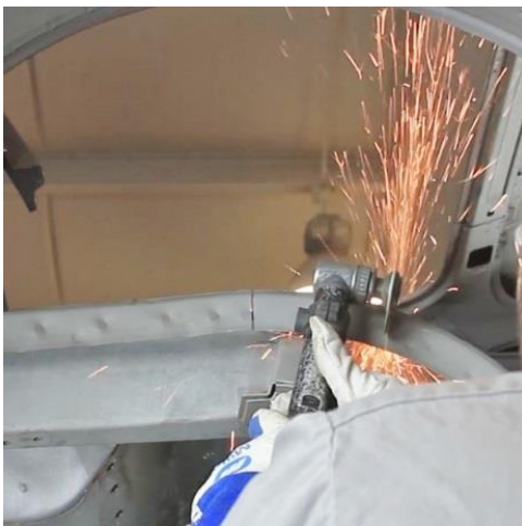
Figure 7 - Remove Flange above Bump Stop Bracket
