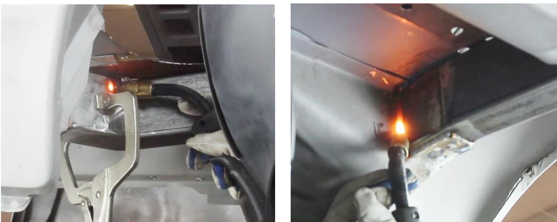
Figure 22 – Weld-In Detroit Speed Frame Rail Section
