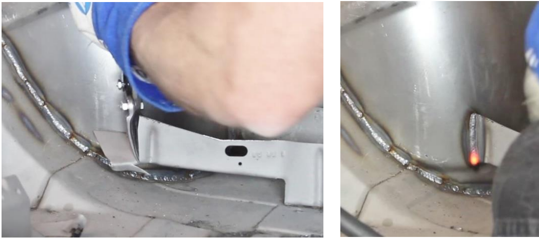
Figure 32 - Re-attach Rear Interior Panel Bracket
