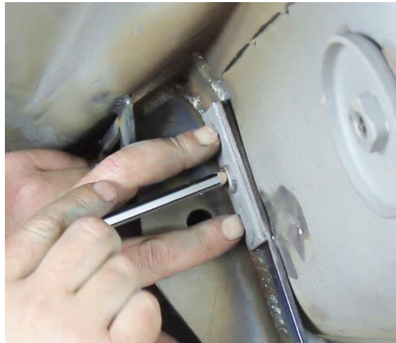
Figure 33 - Re-position the Seat Belt Anchor
