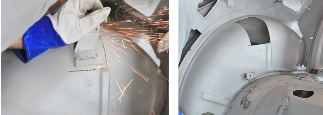
Figure 1 - Remove Lower & Upper Seat Brackets
