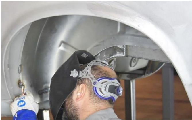
Figure 26 - Weld Mini-Tub to Stock Outer Tub
