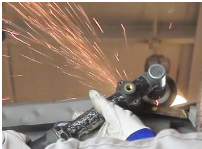
Figure 7 - Remove Flange above Bump Stop Bracket
