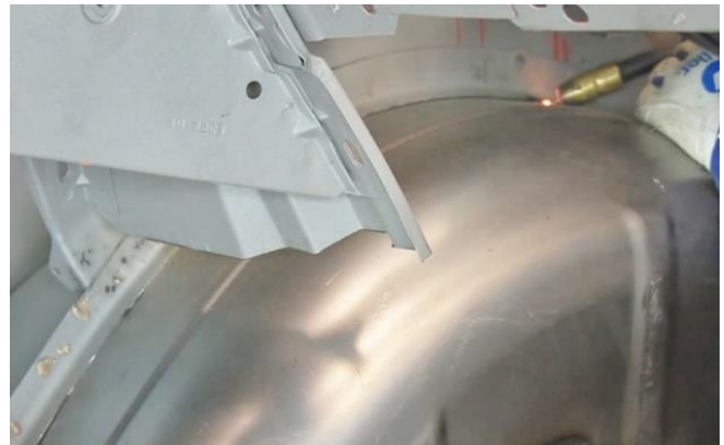
Figure 27 - Stitch Weld Mini-Tub to Frame Rail & Outer Tub Flange
