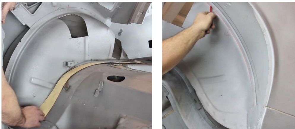
Figure 5 - Trace Floor Pan Cut Template
