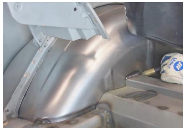
Figure 26 - Weld Mini-Tub to Stock Outer Tub
