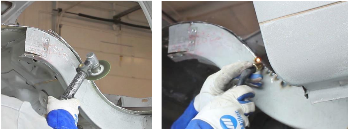
Figure 20 – Cut & Weld Sheet Metal Layers
