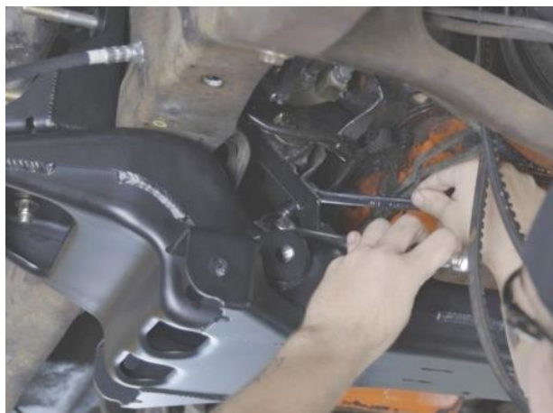
Figure 42 – Install Engine to Brackets
