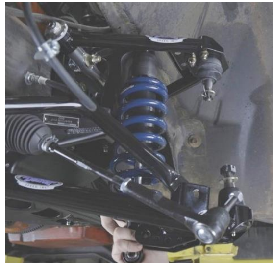
Figure 81 – Position Coilover Shock & Spring Assembly
