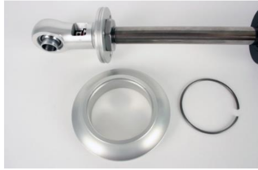
Figure 79 – Upper Spring Seat & Retaining Ring
