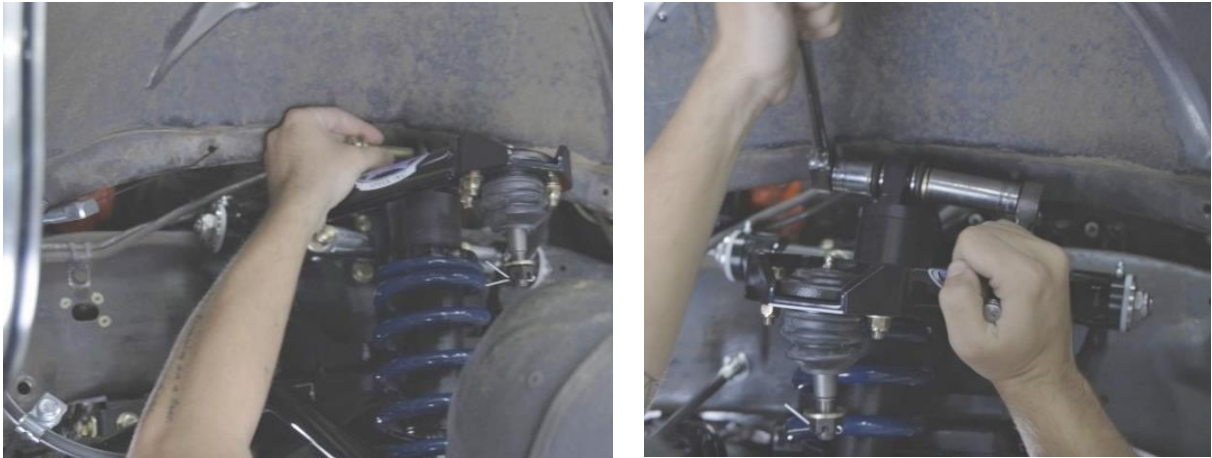
Figure 82 – Install Upper Shock Mounting Hardware
