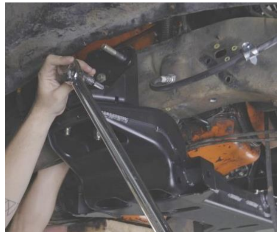
Figure 44 - Torque Cradle Hardware
