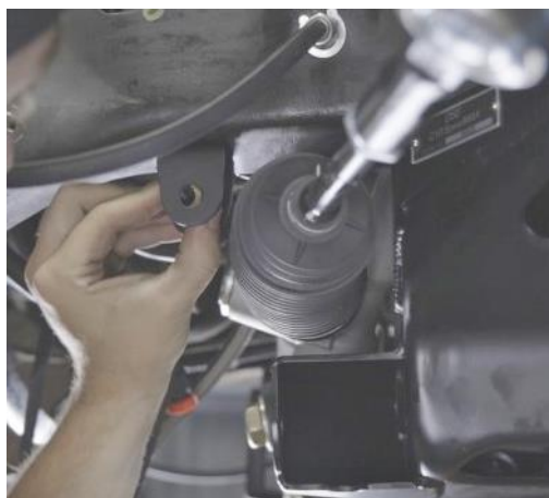
Figure 64 - Install Sway Bar Mount Crush Sleeve
