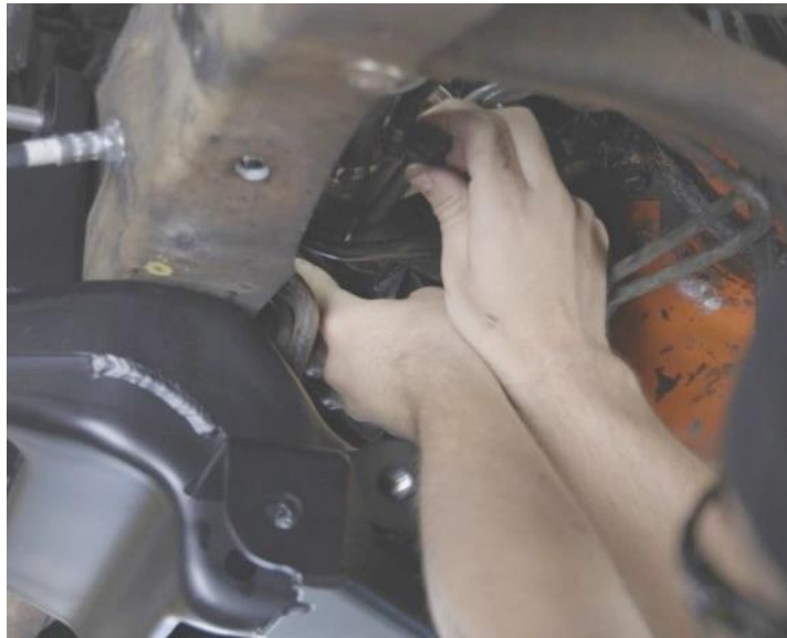
Figure 41 – Install Engine Mounts
