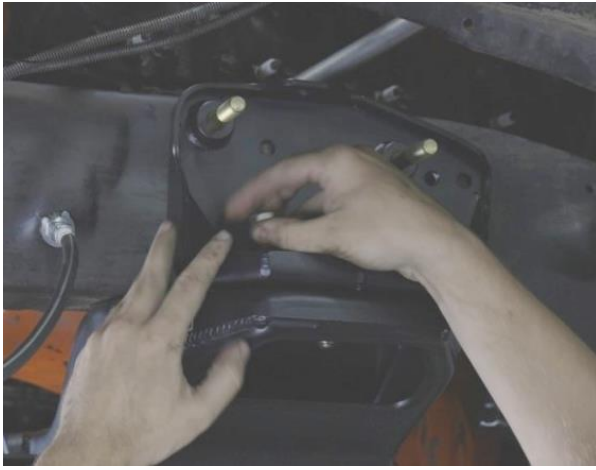
Figure 34 - Loosley Install Upper Control Arm Brackets
