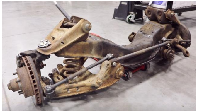
Figure 18 – Remove the Factory Cradle
