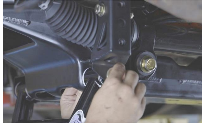
Figure 69 - Tighten Lower Control Arm
