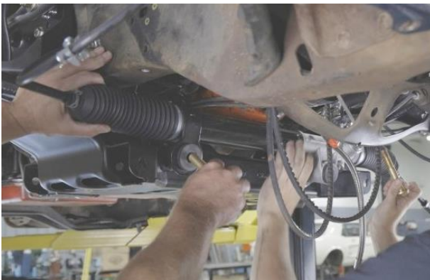
Figure 62 - Install Rack and Pinion
