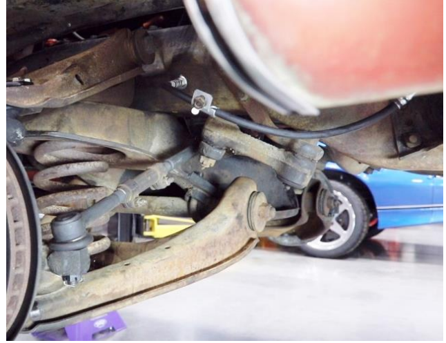
Figure 5 - Remove Brake Hose From Suspension
