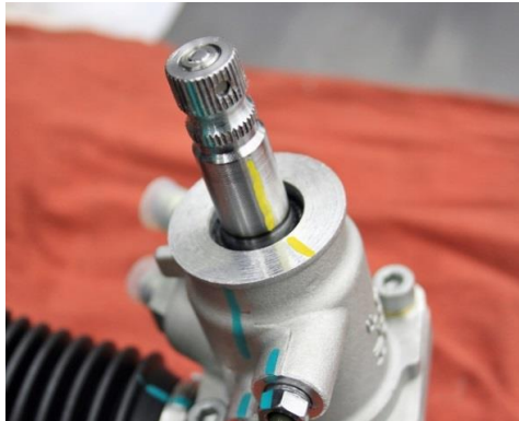
Figure 61 - Center the Rack & Pinion
