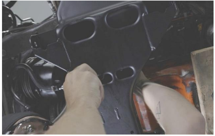
Figure 40 – Install Engine Mount Brackets
