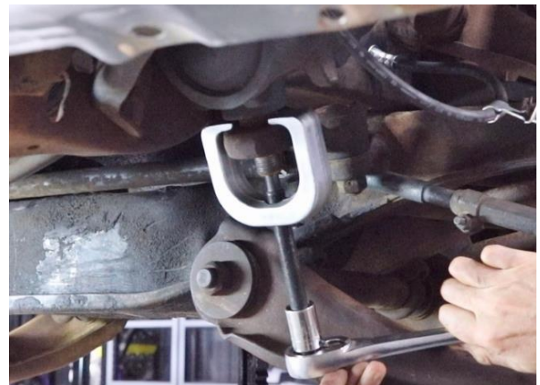
Figure 7 - Remove Pitman Arm
