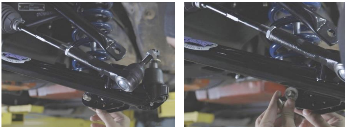
Figure 84 – Install Lower Shock Mounting Hardware
