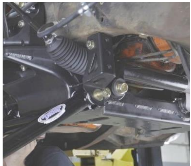
Figure 68 – Install Front Lower Control Arm Hardware
