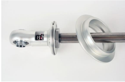
Figure 78 – Remove Upper Spring Seat
