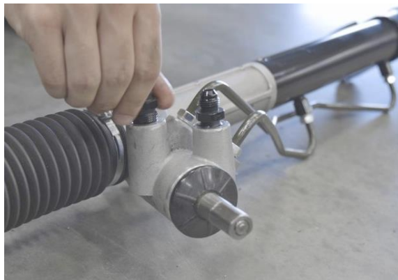
Figure 59 - Install Rack Fittings
