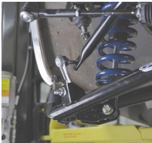
Figure 87 - Install Sway Bar End Link
