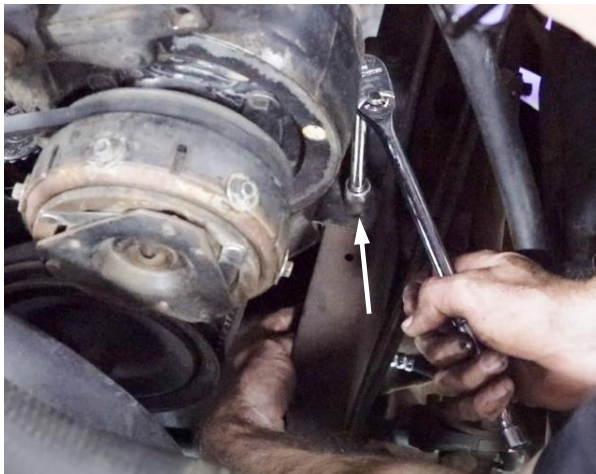
Figure 10 - Remove Upper Engine Bracket Hardware
