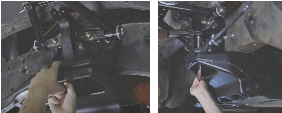
Figure 51 - Torque Upper Coilover Mount
