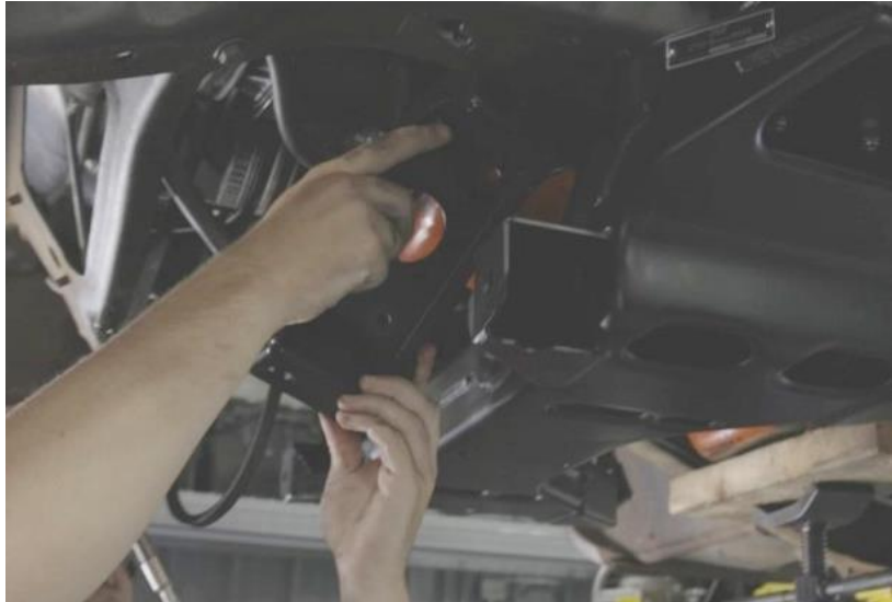
Figure 38 – Position Engine Mount Brackets
