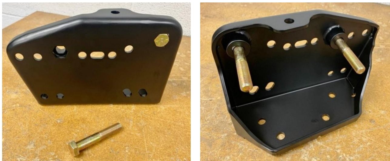
Figure 32 – Install Upper Control Arm Bolts
