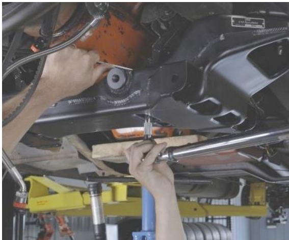
Figure 44 - Torque Cradle Hardware
