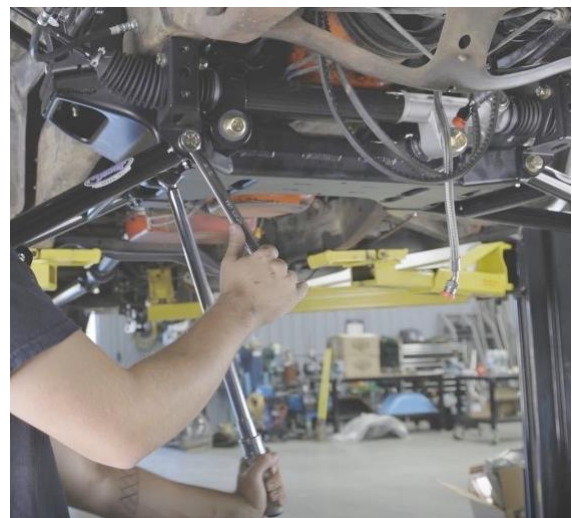
Figure 70 - Torque Lower Control Arm
