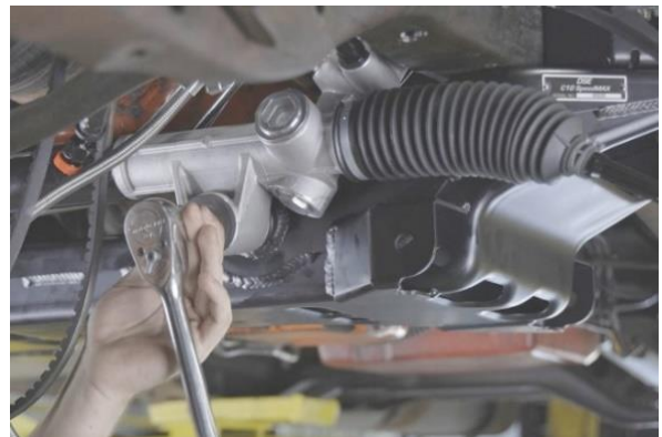
Figure 62 - Install Rack and Pinion
