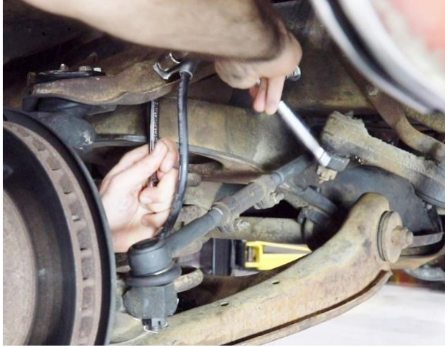
Figure 5 - Remove Brake Hose From Suspension
