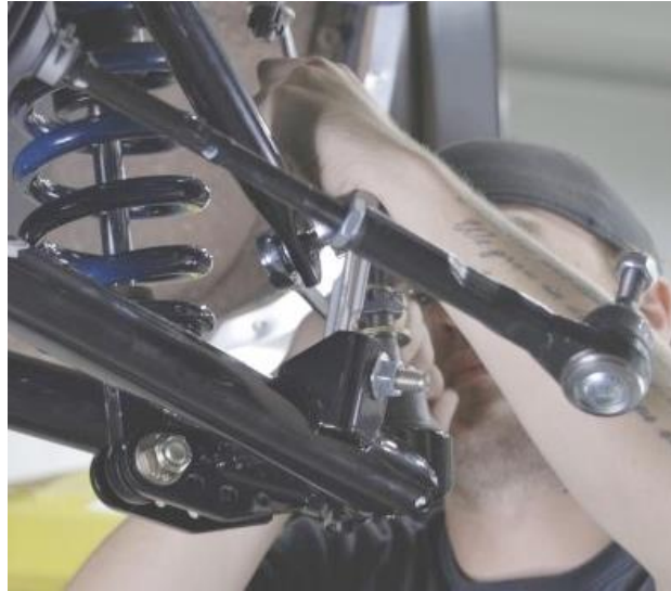
Figure 88 – Tighten Sway Bar End Link
