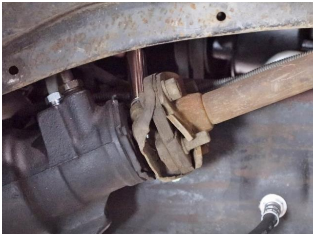
Figure 19 – Remove the Rag Joint
