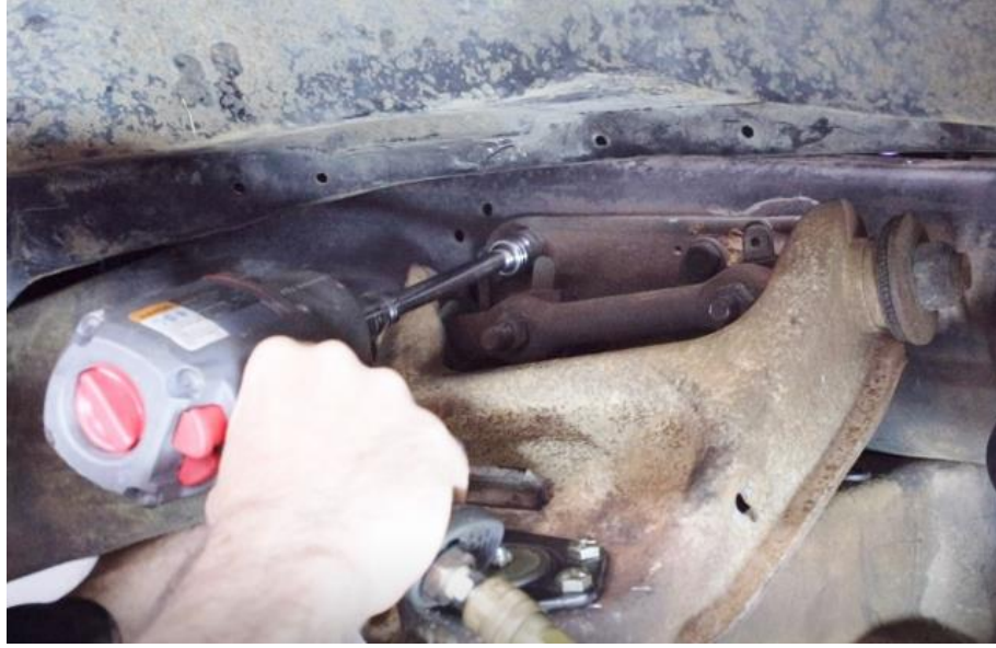
Figure 17 – Remove Upper Control Arm Bracket Bolts
