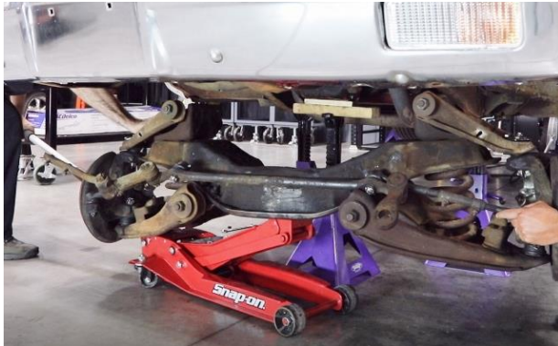
Figure 18 – Remove the Factory Cradle
