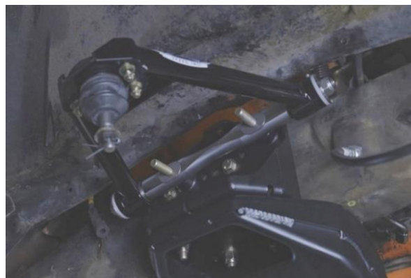
Figure 45 - Install Upper Control Arms
