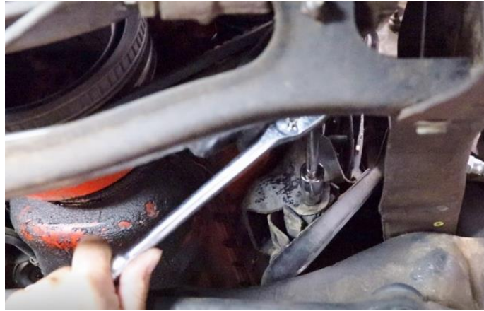
Figure 8 - Remove Engine Mount Hardware
