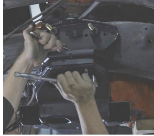
Figure 34 - Loosley Install Upper Control Arm Brackets
