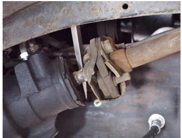
Figure 19 – Remove the Rag Joint
