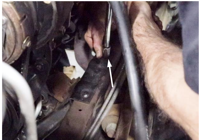
Figure 10 - Remove Upper Engine Bracket Hardware
