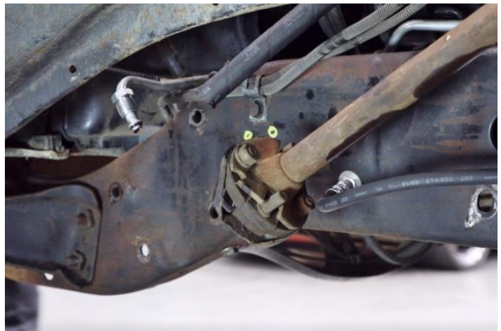
Figure 22 - Remove Steering Gear
