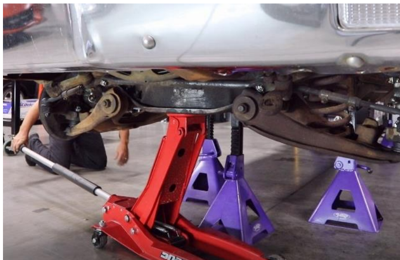
Figure 16 - Prepare to Remove the Cradle
