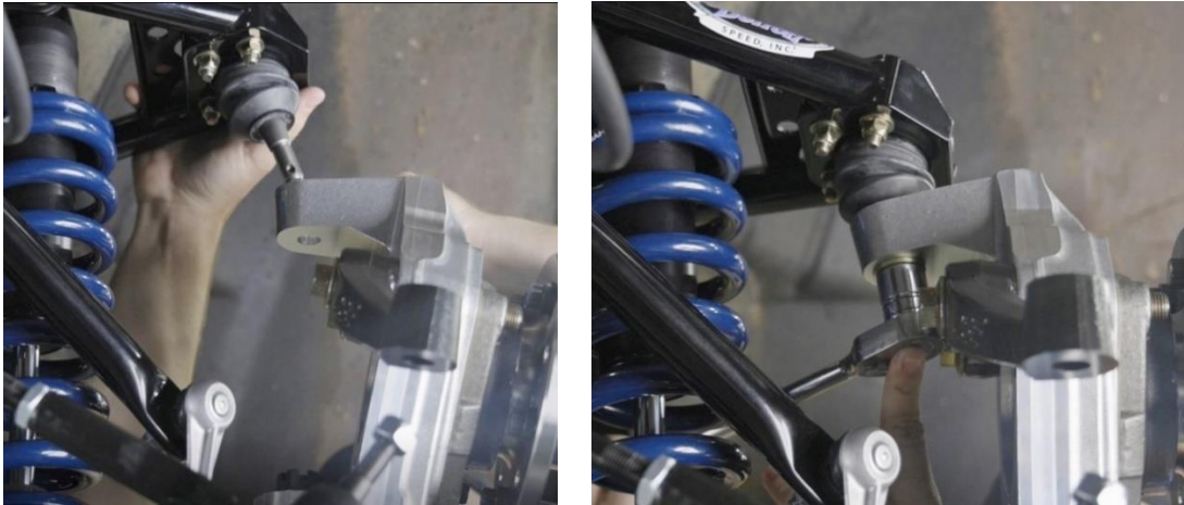
Figure 94 - Install Upper Ball Joint
