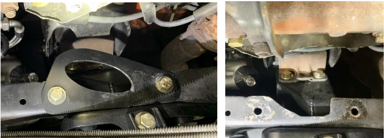
Figure 24 - Notch Frame Rail
