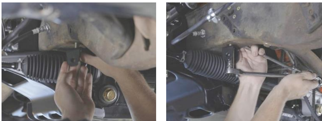
Figure 63 - Install Sway Bar Bracket
