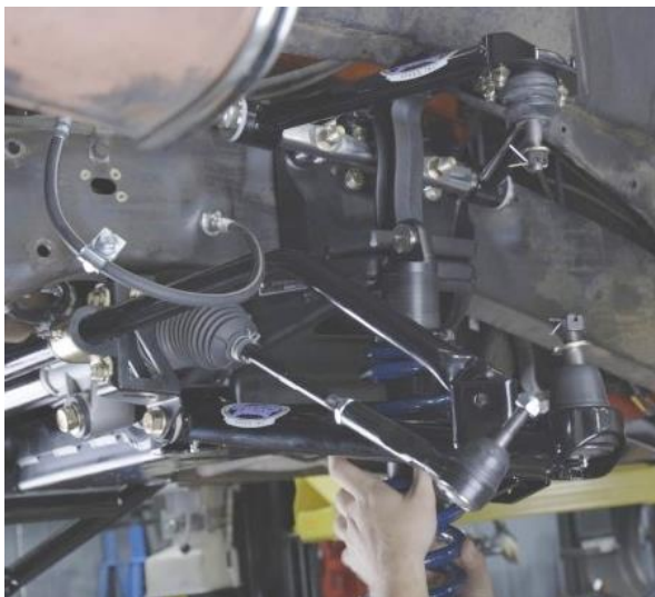
Figure 81 – Position Coilover Shock & Spring Assembly
