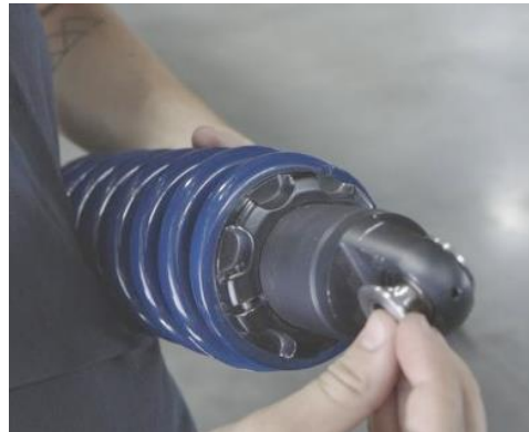
Figure 80 – Install Tapered Spacers
