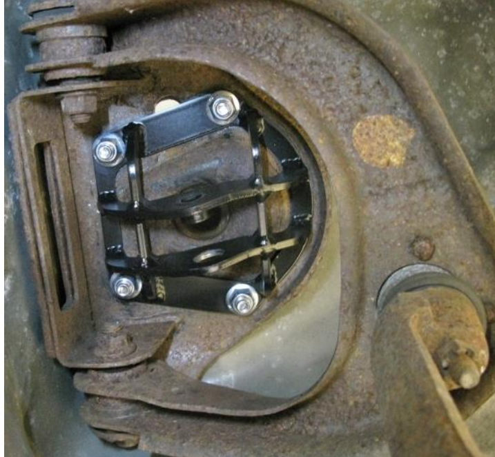
Figure 6 - Install Upper Shock Mount
