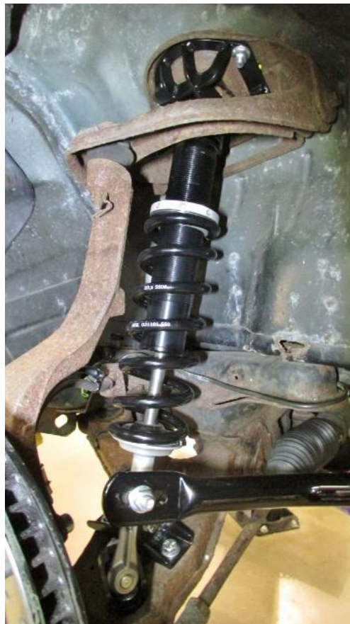
Figure 12 - Installed Coilover Kit
