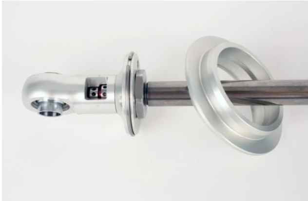
Figure 8 – Removing the Upper Spring Seat
