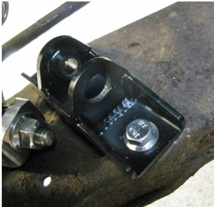
Figure 7 - Install Lower Shock Mount
