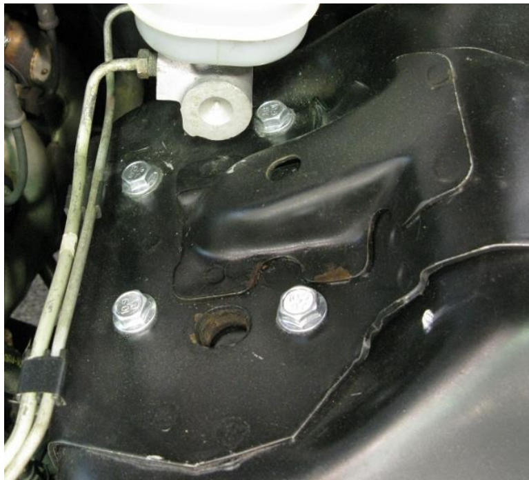
Figure 5 - M10-1.5 x 30mm Flange Hex Bolts
