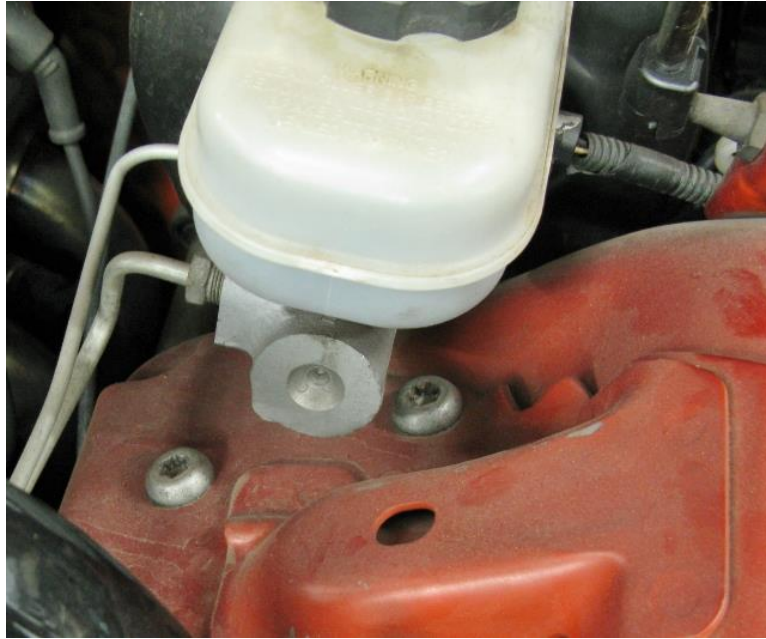
Figure 2 – Remove Torx Bolts
