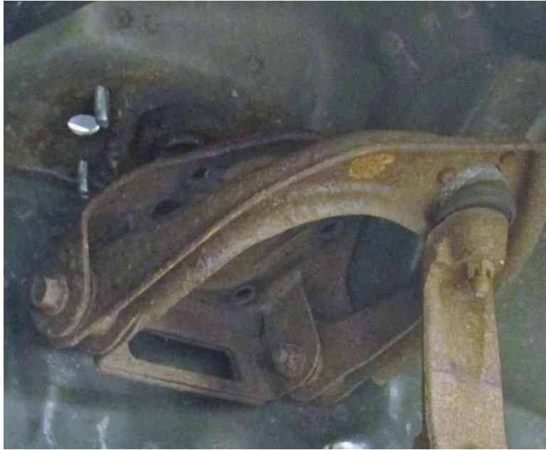
Figure 4 - Drop Upper Control Arm Down
