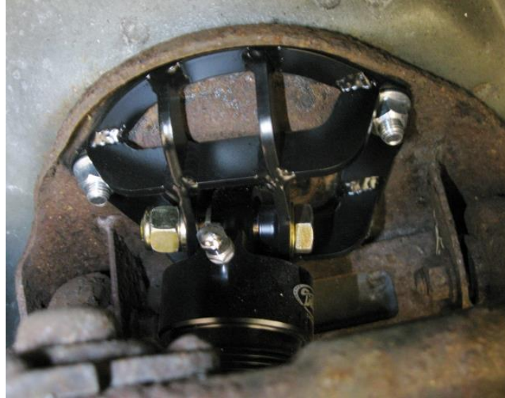
Figure 10 – Install Upper Shock Bolt
