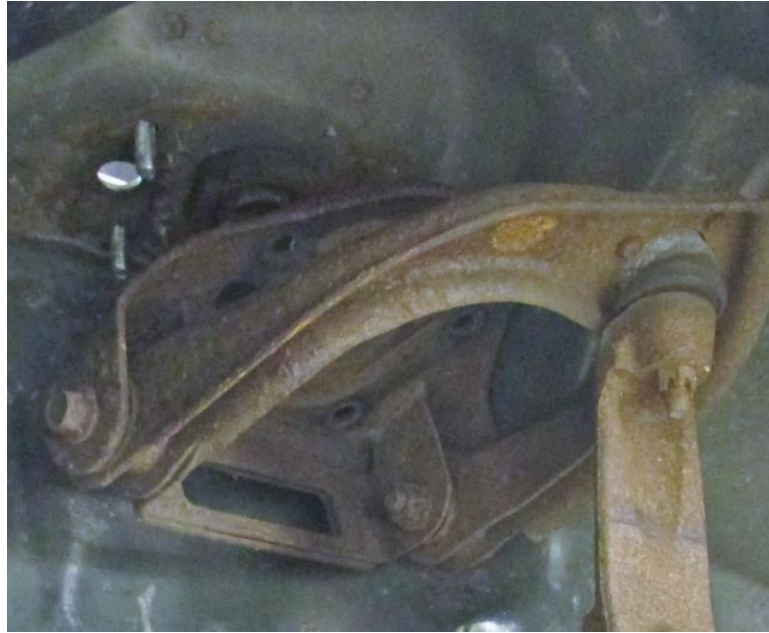
Figure 4 - Drop Upper Control Arm Down
