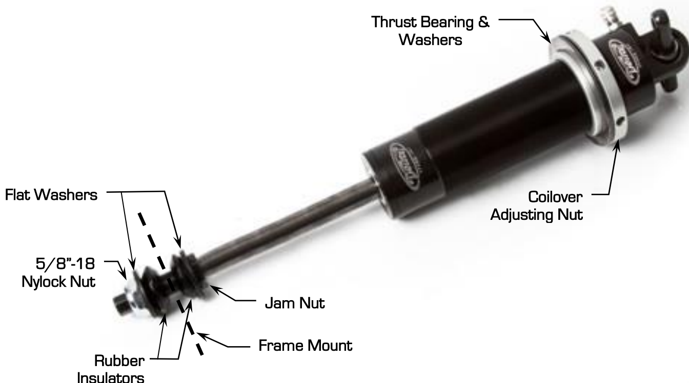
Figure 1 - Shock Assembly
