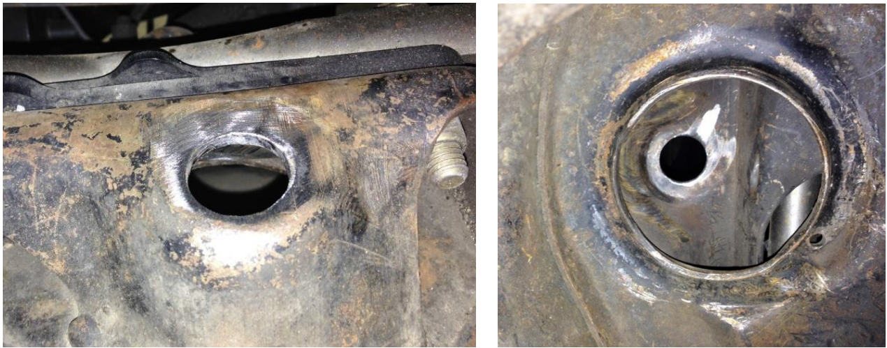
Figure 2 – Remove Sharp Edges/Burrs
