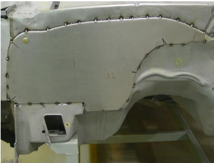
Figure 1 - Panel Tacked in Place
