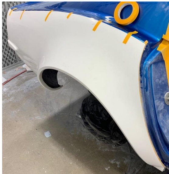
Figure 2c - Fit the Detroit Speed Rear Fender Flares
