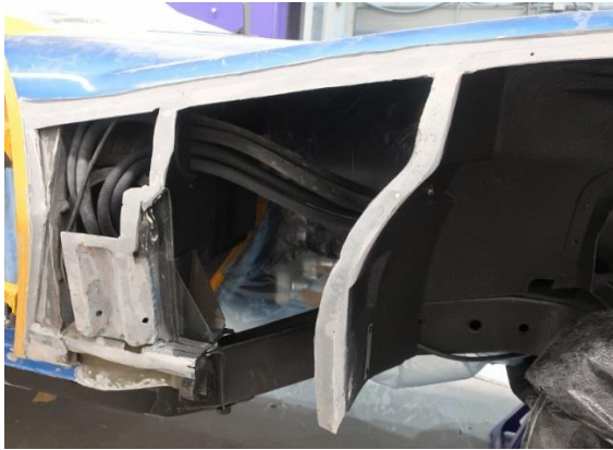
Figure 1a – Remove Front Factory Fender Flares
