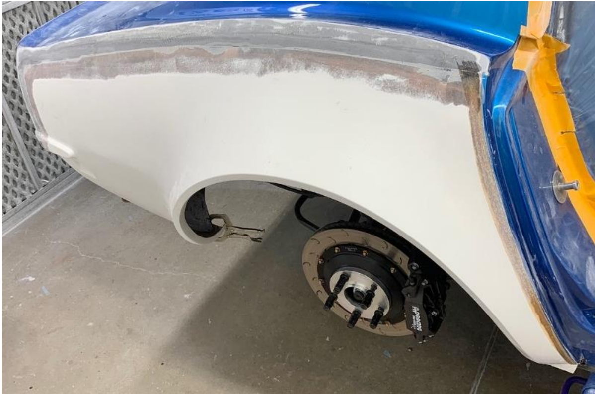
Figure 3 - Fiberglass the Fender Flare to the Body
