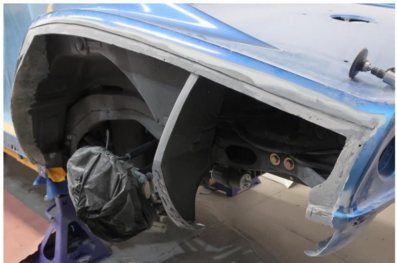
Figure 1b – Remove Rear Factory Fender Flares
