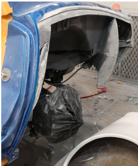
Figure 1b – Remove Rear Factory Fender Flares
