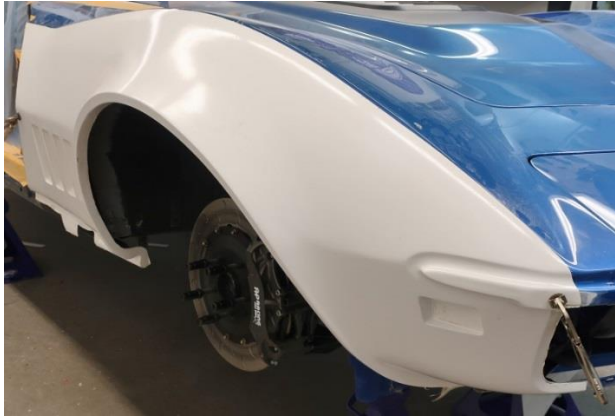
Figure 2a - Fit Detroit Speed Front Fender Flares
