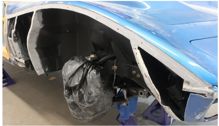
Figure 1a – Remove Front Factory Fender Flares
