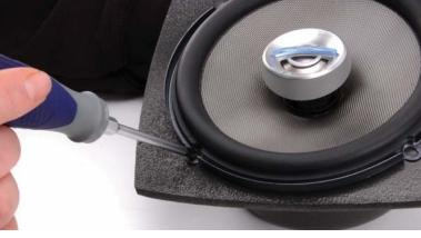
2. Perforate screw holes using and awl or other pointed tool. Use care not to tear the baffle material.
