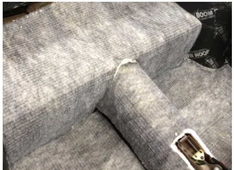
UC Lite installed with gray side up.
