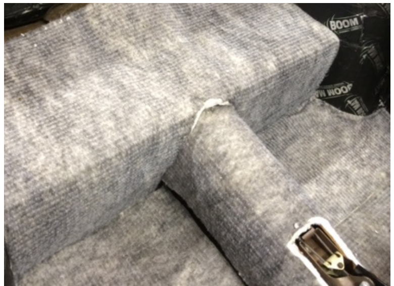
UC Lite installed with gray side up.
